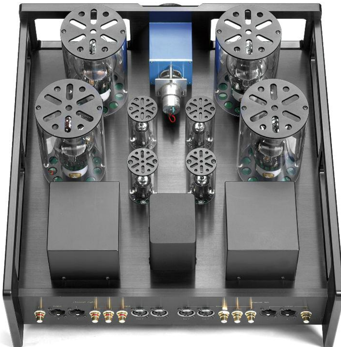
Prodigious: What looks like an integrated amplifier with its four 300B valves is in fact a preamplifier – albeit one that could easily drive a high-impedance 16 Ohm loudspeaker
